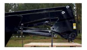
Place a piece of wood (or rubber pin locking) between the parallel link and the arm before knocking out the middle pin. Pivot the bearing box backwards and reinsert the pin in the hole in the bearing box so that the pin acts as a wedge. Replace the bushings and refit the middle pin.
