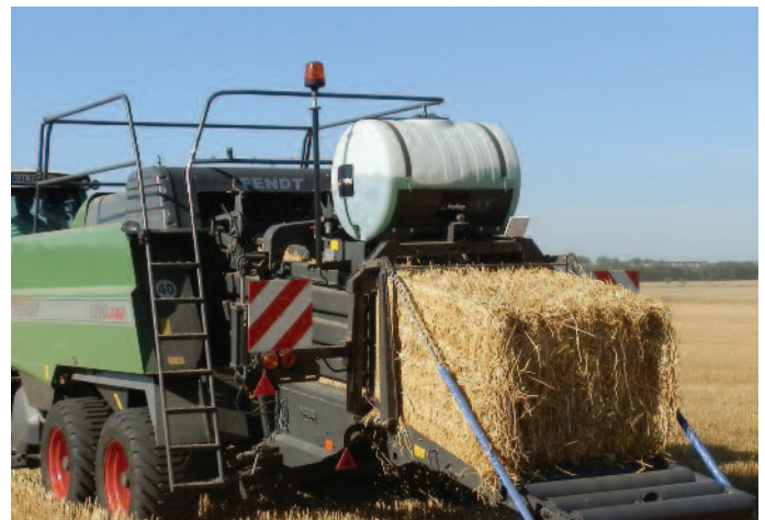
400 or 420 litre tank with three pumps for large square balers
