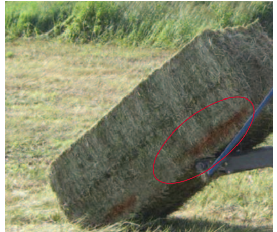
A hay bale marked when the alarm was set to 27%, showing the middle section is within the preferred moisture range, while the end flakes were above 27% moisture.
