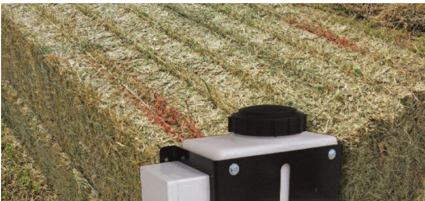
A hay bale marked when the alarm was set to 27%, showing the middle section is within the preferred moisture range, while the end flakes were above 27% moisture.
